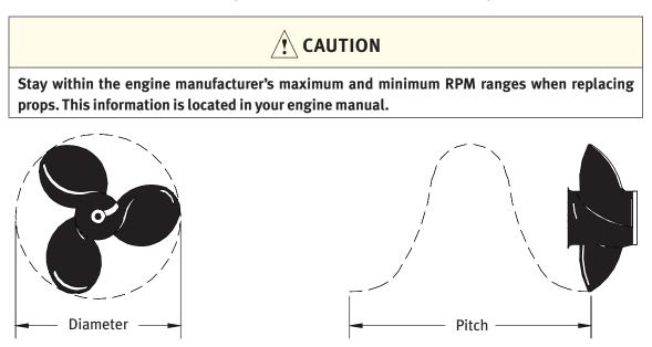
Diameter and pitch are the two basic dimensions of a propeller. Diameter is the distance across the circle made by the blade tips as the propeller rotates. Pitch is the theoretical (not accounting for slippage) forward distance the propeller would move in one revolution. An example of a propeller dimension would be 14 X 17 for a propeller having a diameter of 14 " (35.6 cm) and a pitch of 17 " (43.8 cm).
